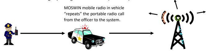
P25, dual-band portable on FCC licensed frequencies. Linked to the MOSWIN mobile radio in the vehicle via a repeater.
